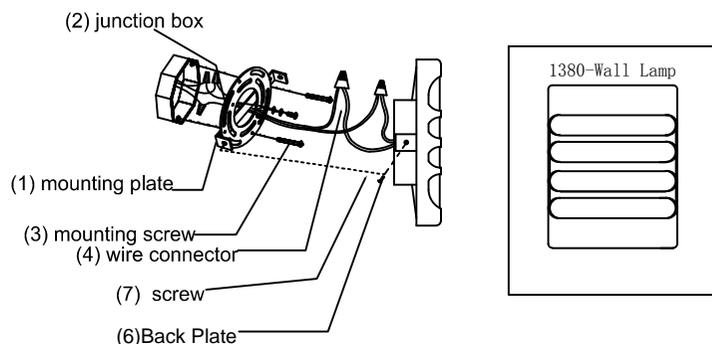
1. Remove the screw (7) and then take out the back plate (6).
