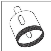
**Diamond 35mm hole saw (for faucet hole trimming)**
