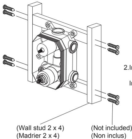
2. Install the horizontal 2 x 4 between the studs.
