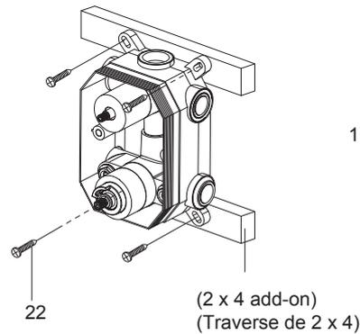
1. Install the faucet on the horizontal 2 x 4 add-on to fix the faucet between the studs.
