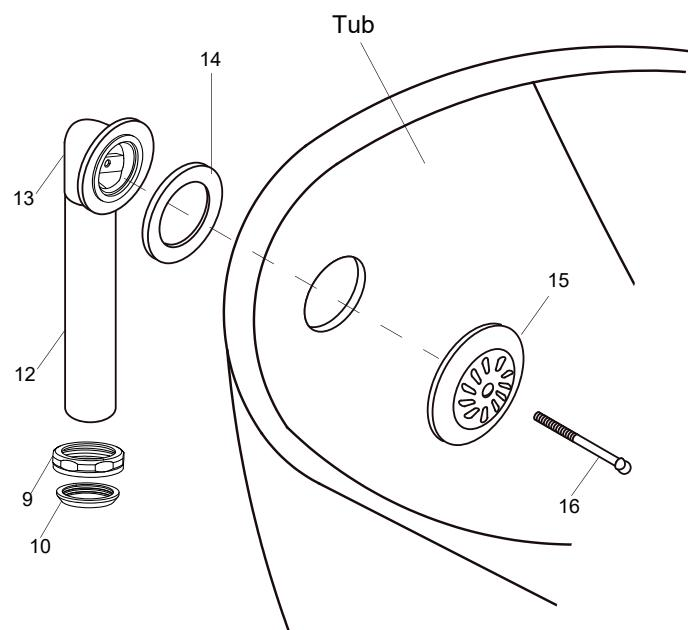
1. Install the overflow drain pipe into the overflow hole.
