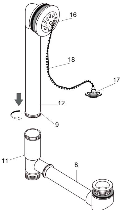
3. Connect overflow hole pipe and the "T" pipe#11.
