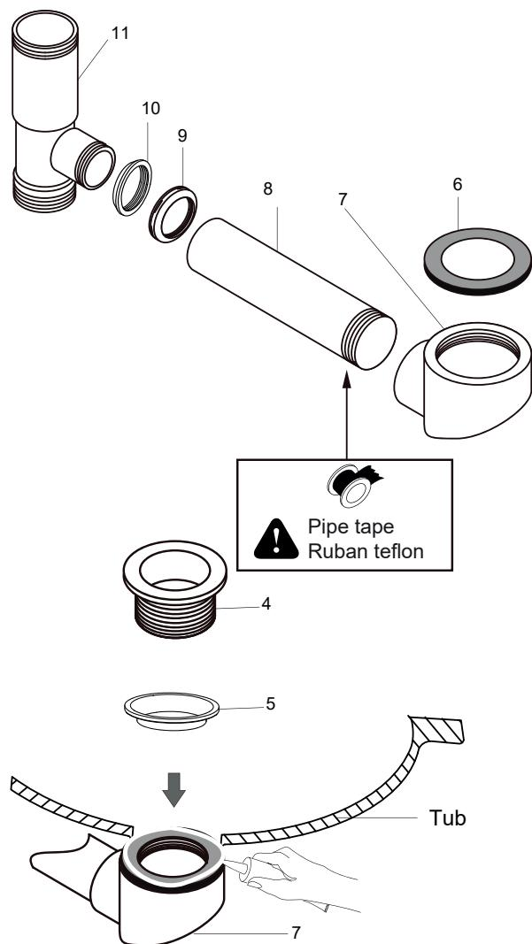
2. (A) put the drainer onto the tub drain hole.
