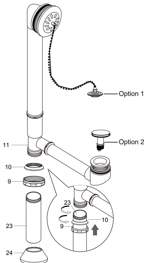
4. Put the 6" straight pipe with the overflow hole pipe. and put on the decoration flange.
