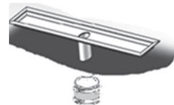
En: Join AlinO Linear Drain with 2" No Hub Coupler. Measure the distance between drain and the pipe, cut a small piece of 2" pipe to join (if required) by using ABS/PVC solvent. Apply modified thin set mortar on the substrate, and position drain body support and then drain body.
