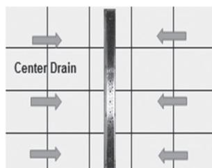
En: **Center drain application:** Measure distance from each wall to determine drain location. Cut Tray to fit or add AlinO Linear Extensions kit, if required.
