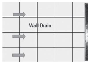
En: **Wall drain application:** Center of drain hole should be 2-1 / 4" from expected finished wall surface.
