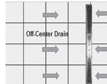
En: **Off-Center drain application:** Measure distance from the wall to the center of the drain, and deduct 2.5" for drain body support and cut Off-Set Tray (27.5" x 36").
