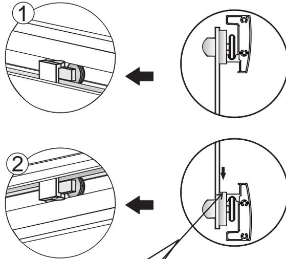
**!** Clip the bottom of the door in the bottom rail. The rollers are pressed down to allow the rollers clip to be into the rail.
