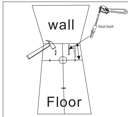
4. Install the foot bolt and nut set into the floor drilled holes until no screw thread can be seen.
