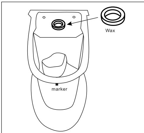
5. Installed the wax onto toilet bottom drain hole
