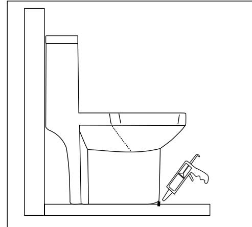
8. Applied silicon glue to the slot between toilet bottom and floor
