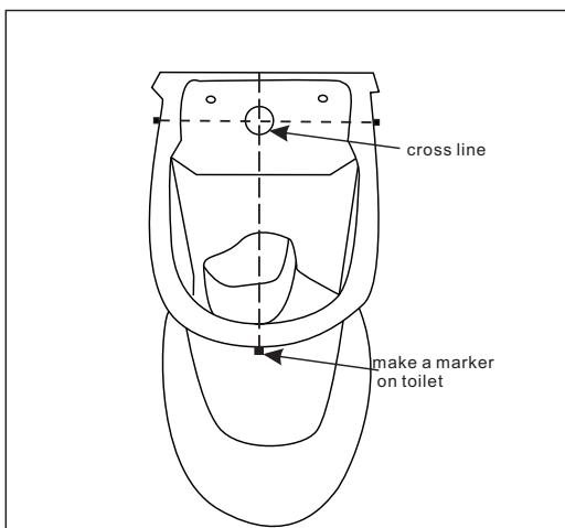
1. Marked the cross lines under toilet bottom, measure the distances between toilet bottom drain hole center to the front and 2 sides. (make a marker on toilet front)
