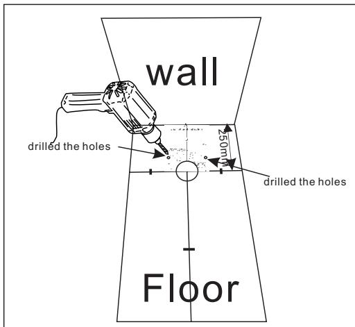
3. According to «toilet foot bolt installation drawing», drilled the holes on the floor for bolt as drawing attached.
