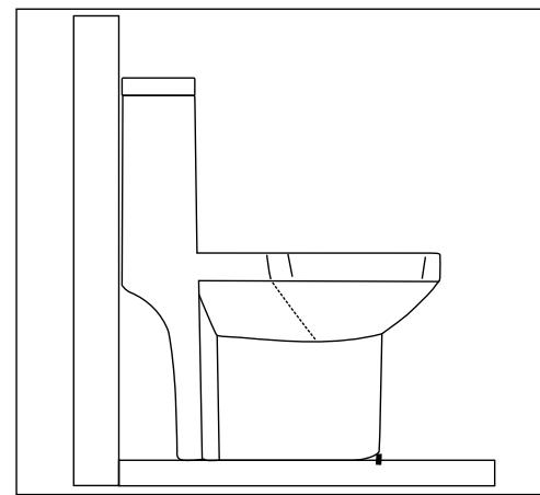
6. Placed the toilet to the floor follow 3 already marked on step points 1, 2 and 3 on floor.
