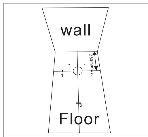
2. According to step 1 distances measured, marked 3 points on the floor, as point number 1, 2 and 3 for installation later.
